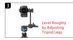
Set up the Nodal Ninja. Mount the camera. Then roughly level (bubble inside or on the circle line) it by adjusting the length of tripod legs. This prevents the leveler from going out of adjustment range.
