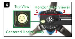
Stand in a position so that 2 rollers (**1** and **2**) are horizontal in front of you. Look at the bubble from vertically above. Adjust the horizontal rollers to center the bubble horizontally.
