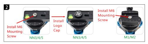
Align the anti-twist plate/ sockets and place the lower rail or QRC-55/65 on RD3L. Install and tighten the M6 mounting screw using a 4mm hex key. For NN3/4/5, install the logo cap on the mounting screw. Now the Nodal Ninja with RD3L is ready for use.
